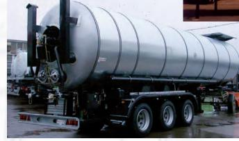
Select from the most varied heating systems and laggings up to 100 mm, which allow for a transport of bitumen up to 250°C.
