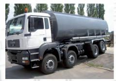
With a tank volume for truck bodies from 4,000 I to 30,000 I and of 20,000 I to 60,000 I for semi-trailers, our vehicles can be used to transport diesel, fuel, kerosene, crude oil or heavy oil depending on their design. As a matter of fact our tanks are manufactured in accordance with the ADR directives.
